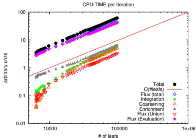
Computational time (per time-iteration) as a function of the stochastic discretization (total number of leaves) ; left :  $N_0 = 2$  and  $\eta = 10^{-3}$  ; right :  $N_0 = 3$  and  $\eta = 10^{-4}$ .
