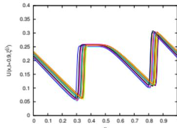
20 realizations of the initial condition (left) and solution at  $t = 0.4$  (middle) and  $t = 0.9$  (right) : 2 shocks and 2 rarefaction waves.
