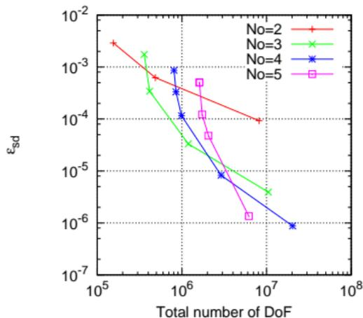
Left : error as a function of the total number of leafs in the final discretization ( $t^n = 0.5$ ). Right : error as a function of the total number of degrees of freedom (number of leafs times the dimension of the local polynomial basis).
