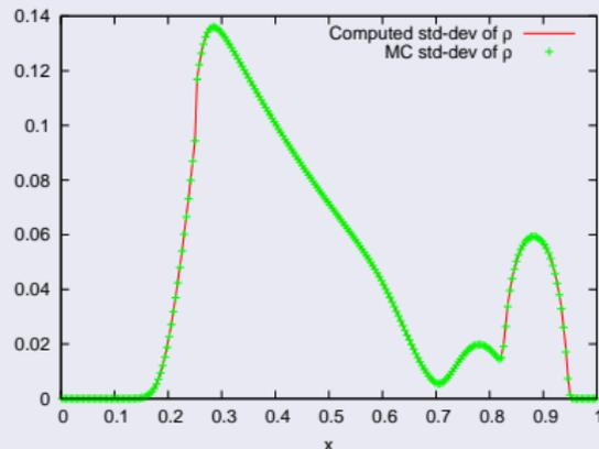
Comparison of mean and standard deviation of density at  $t = 1$ , computed with Galerkin (using  $N_r = 3$  and  $N_o = 2$ ) and MC methods
