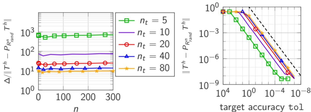
Figure: Convergence behavior of adaptive algorithm (left) and effectivity of a posteriori error estimator  $\Delta / \|T^h - P_{R_{rand}^n} T^h\|$  (right) for increasing number of test vectors  $n_t$ .
