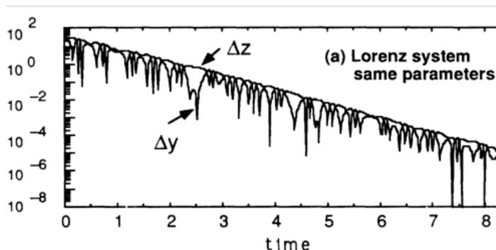
**Figure:** Synchronization between two copies of the Lorenz '63 model, coupled through the  $x$ -variable. The differences  $\Delta y := |Y - y|$  and  $\Delta z := |Z - z|$  decay exponentially in time. Note that even in this chaotic model, adding more data from the  $x$ -coordinate time series helps for convergence.
